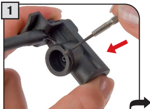
1 Remove the O-ring with a pointy object.
