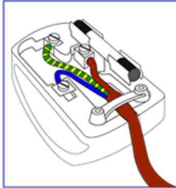
**2. The BLUE wire must be connected to the terminal which is marked with the letter "N" or coloured BLACK.**
