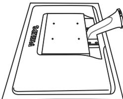
2. Hold the monitor base stand with both hands and firmly insert the base stand into the base column.
