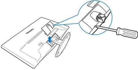
2. Remove 4 screws and then remove the base from the monitor.
