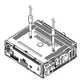
Remove the mounting sleeve with the supplied disassembly tools.
