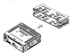
Install the sleeve into the dashboard and hend the tabs outward to fix the sleeve
