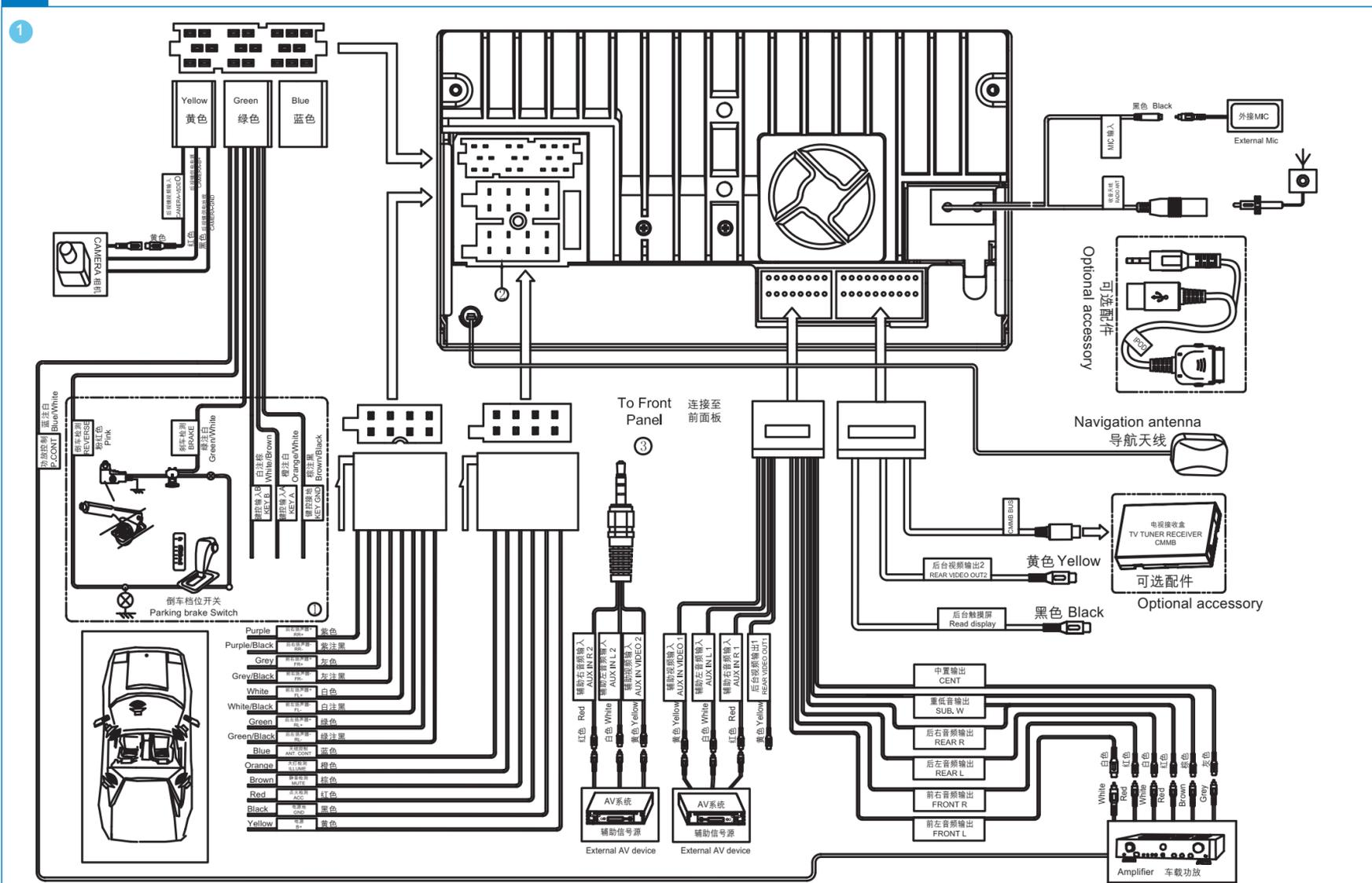
Remark: ③ Here connect the external AV device to the AV IN socket on the front panel of the car audio system. 备注: ③此处AV IN线与前面板AV IN接口相接
