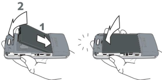
4. Replace the battery cover: slide it until it clips.
