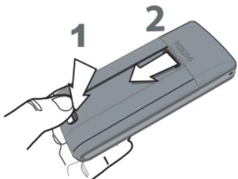
2. Slide the SIM card in its slot (make sure that the clipped corner is in the correct place and the connectors are facing the phone) then replace the holder.
