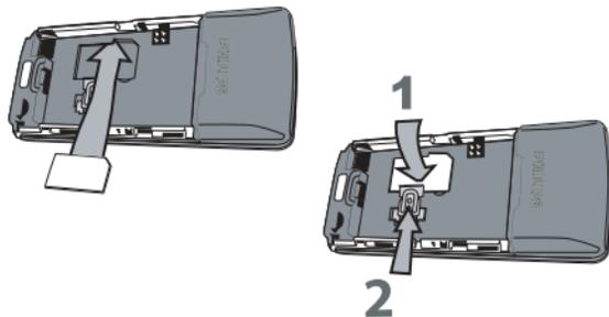
3. Insert the battery (make sure that the connectors are facing the connectors of the phone) and press until it clips.
