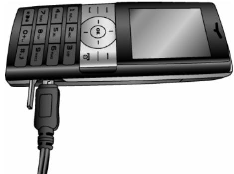
The battery symbol indicates the state of charge. During charging, the charge indicators will scroll; it takes around 4 hours to fully charge the battery. When all the scroll bars are steady, the battery is fully charged. You can then disconnect the charger. Depending on the network and condition of use, talk time and stand-by time can go up to 17 hours\* and 1440 hours (2 months)\* respectively.
