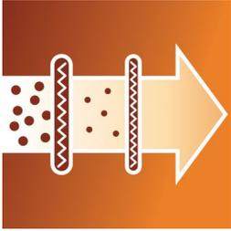
The two stage filtration system ensures that, once inside, the dirt cannot escape again. The first filter blocks most of the dirt, while the second filter traps the finer dust particles.
