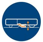
The robot vacuum cleaner comes with a movable nozzle that follows the contours of the floors, carpets, rugs, etc. to ensure accurate cleaning results.
