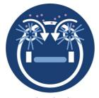
First two long brushes swipe dirt and dust into the path of the robot. Then, the nozzle picks up dirt and dust thanks to its powerful motor.
