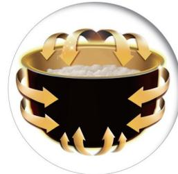
There is heating system surround the multicooker, including heater assembly on the top, heater assembly all around and main heater assembly on the bottom, 3D heating system for even heating, more effective warm keeping and better baking result
