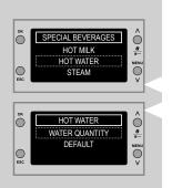
2 Select HOT WATER by pressing the "√" or "∧" scrolling button. Press "**OK**" to confirm.
