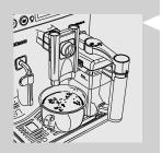
4 The machine starts pouring hot milk. The pouring can be stopped earlier by pressing the "ESC" button.
