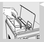
5 Open the lid and remove the water tank by the handle.
