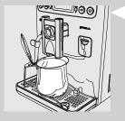
16 Place a container under the dispensing spout to catch the small amount of water which will be dispensed.
