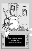
6 Place a container (1,5 lt) under the coffee dispensing spout. Press the "**OK**" button to start the cleaning cycle.
