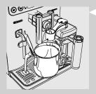
**IS** Empty the container and place it back under the coffee dispensing spout. Open the milk dispenser by turning it clockwise.
