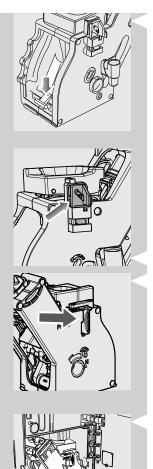
8 Gently pull down the lever until it is in contact with the brew group base and the two reference signs on the side of the brew group do match.
