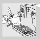
5 When the dispensing has finished, empty the container and place it under the hot water/steam wand.
