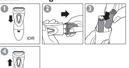
NOTE: Make sure the (+) and (-) markings on the ends of the batteries match those inside the battery compartment.
