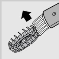
**4** Slide the shaving heads out of the retaining frame and clean them one by one.
