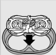
**7** Slide the shaving heads back into the retaining frame and put the retaining frame back into the shaving unit.
