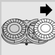
**3** Remove the retaining frame by pushing the sides of the central spring towards each other (1) and lifting the retaining frame out of the shaving unit (2).
