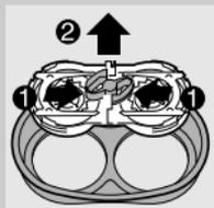
**2** Press the release button (1) and remove the shaving unit (2).
