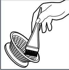
**3** To clean the sieve, use a soft brush. Be careful of the sharp shredders located on the bottom of the sieve. Do not use a metal brush. Allow sieve to air dry thoroughly.
