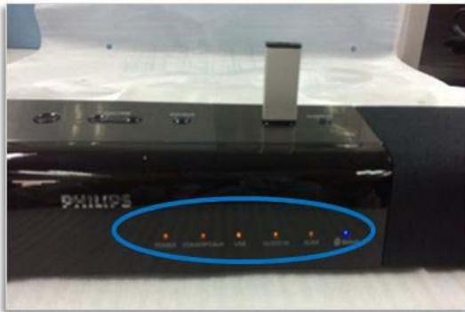
v. After about half a minute, the LED indications flash twice. The product automatically switches to COAX/OPTI/AUX mode. Firmware upgrade is completed.
