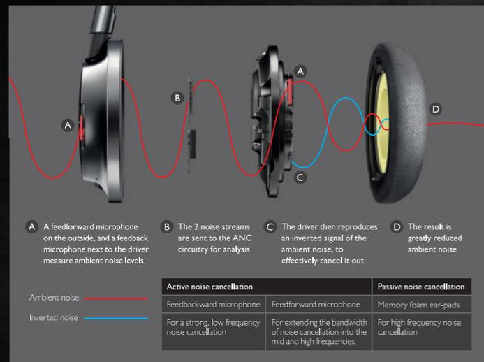
What sets the Fidelio NC1 apart from the competition is its hybrid Active Noise Cancellation (ANC) proficiency. The NC-1 uses a feed-forward and feed-backward ANC solution, which features 4 microphones implemented inside and outside the ear cans that capture noise for advanced processing. This combination ensures cancellation over a wide yet deep frequency range for optimized music enjoyment in any environment.
