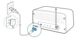
Connect the AC power cord to the **AC MAIN~** socket and then to the wall outlet.
