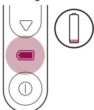
When the battery is almost empty, the charging light lights up orange continuously.
