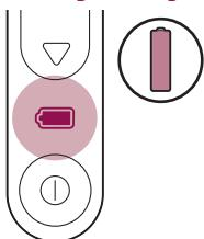
When the batteries are fully charged, the charging light lights up solid green. Fully charged batteries provide at least 370 flashes at light intensity 5.
